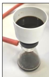
Figure 6: Filtration through a glass fiber filter using a vacuum (shown as an example for a coffee sample)
