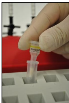
Figure 8: The column is placed into a collection tube before eluent is added, and then the column is centrifuged to remove residual liquid.
