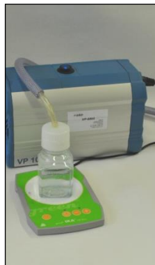
Figure 9: Setup for degassing the reaction buffer (aokinReactionBuffer). This consists of: vacuum pump (hose and vacuum trap, not shown) and the reaction buffer in a bottle with a magnetic stirrer rod on a magnetic stirrer plate.
