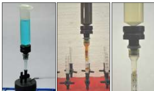
Figure 7: Attachment of reservoir, aokinCadapter and aokinImmunoClean M column to the aokinVacuumAdapter (left), to the vacuum manifold with a coffee sample (middle), and the coffee column after washing with aokinCWash or aokinCWashTween and PBS (right).
